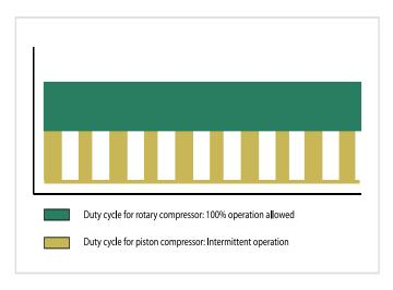
FIGURE 2: Duty cycle comparison between rotary and piston compressors.
