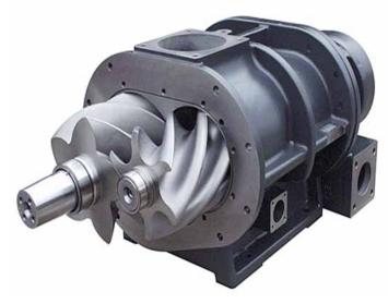
**FIGURE 4:** Rotary screw compressors have a higher initial purchase price, but can be a long term cost effective solution.
