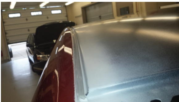
Replacement Roof Division Channel Sealer
